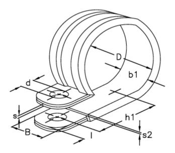
$\begin{array}{lll} b1 & = 15.0 \\ d & = 5.3 \\ Diameter D = 9 \\ h1 & = 12.5 \\ I & = 5.0 \\ s & = 0.50 \\ s2 & = 1.2 \\ Width B & = 12 \\ \end{array}$
